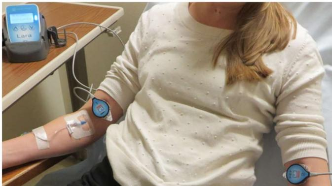
Figure 1. Photo of the injection monitoring system used on a nuclear medicine patient.
